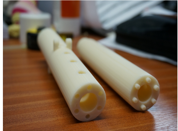
Figure 6: A 3D-printed Clarinet before having keys assembled. The instrument is constructed in 4 quarters split dorsally to facilitate the removal of filler material and transversely so that it can be produced by the small prototyping printer at The University of Glasgow's engineering workshop.
